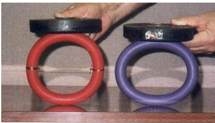
Fig. 1: Comparison of the deformations of two rubber rings
